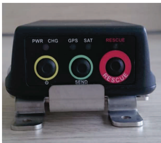
SmallTrack correctly inserted in the bracket.
