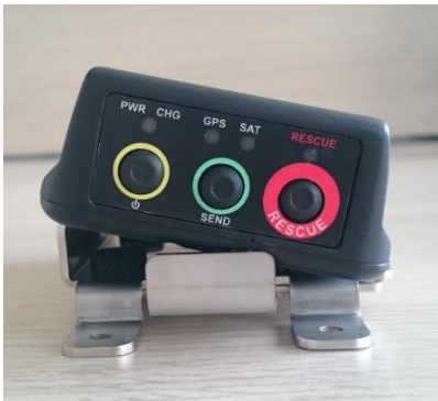
Push the SmallTrack in the bracket
