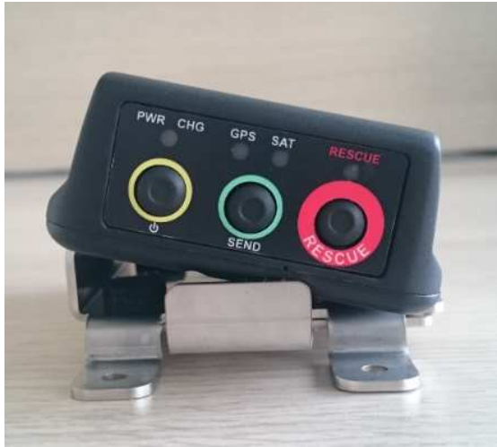
Push the Smalltrack in the bracket
