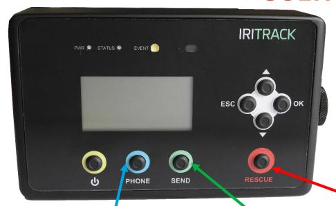
Buttons must be pushed until the LED « STATUS » flashes and the sending indication on the screen (1 second).
