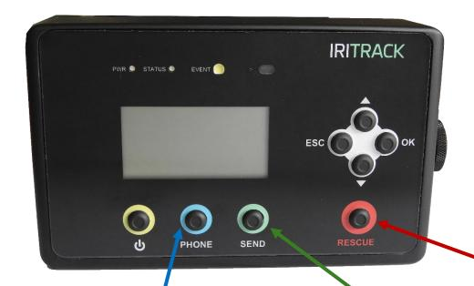
Buttons must be pushed (3 seconds) until the LED « STATUS » flashes and sending indication pops on the screen.
